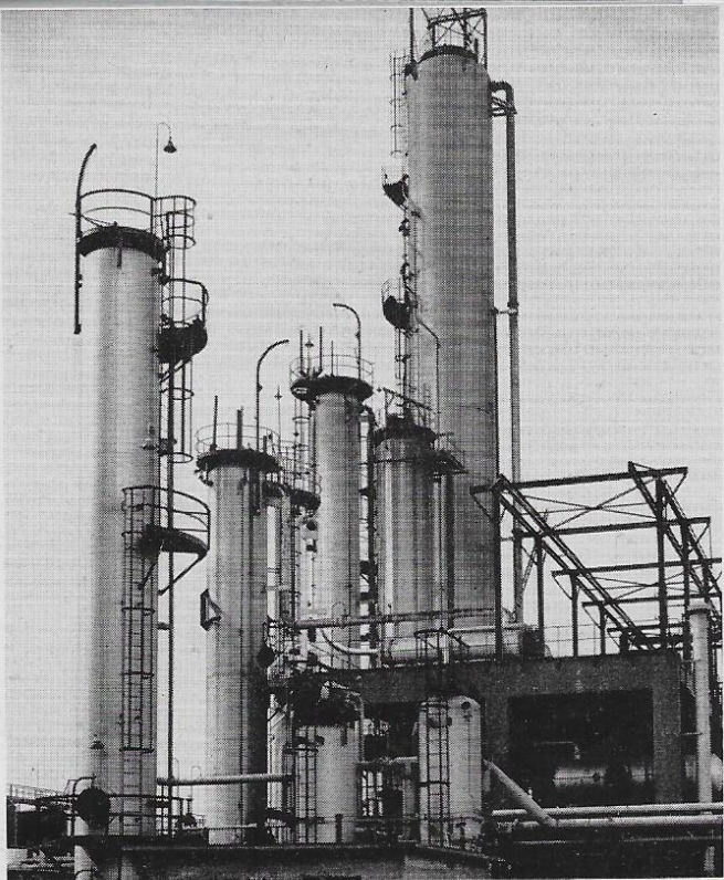
Hydrogen sulfide is first absorbed from fuel gases by DEA solution in the Unit 110 absorption tower, left . . .
